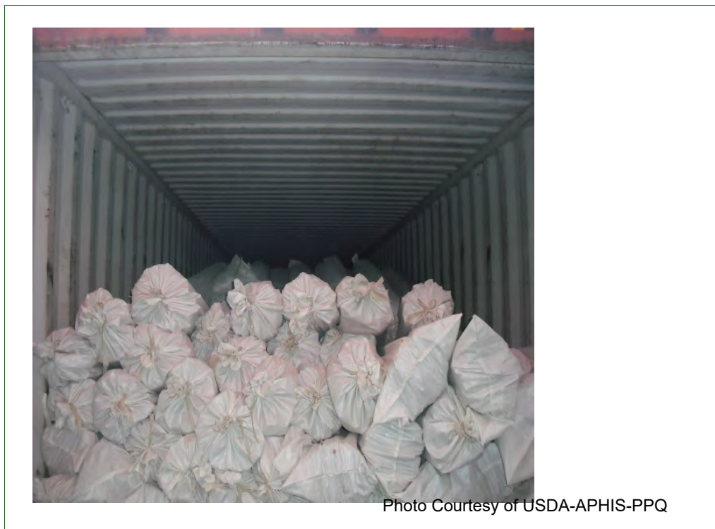
Figure 5-5-3 Example of Adequate Space Above Bamboo Bundles
