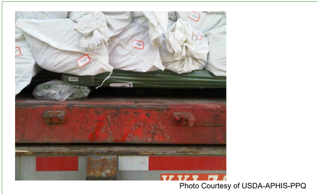
Figure 5-5-2 Example of Inadequate Spacing Under Bamboo Bundles
