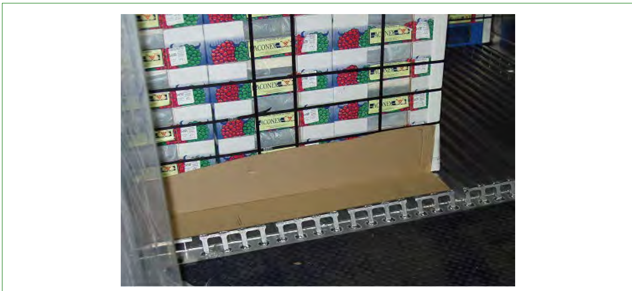
Figure 3-7-5 Proper Placement of Cardboard Between the Last Pallet Row of Fruit and the Back Doors of the Container
