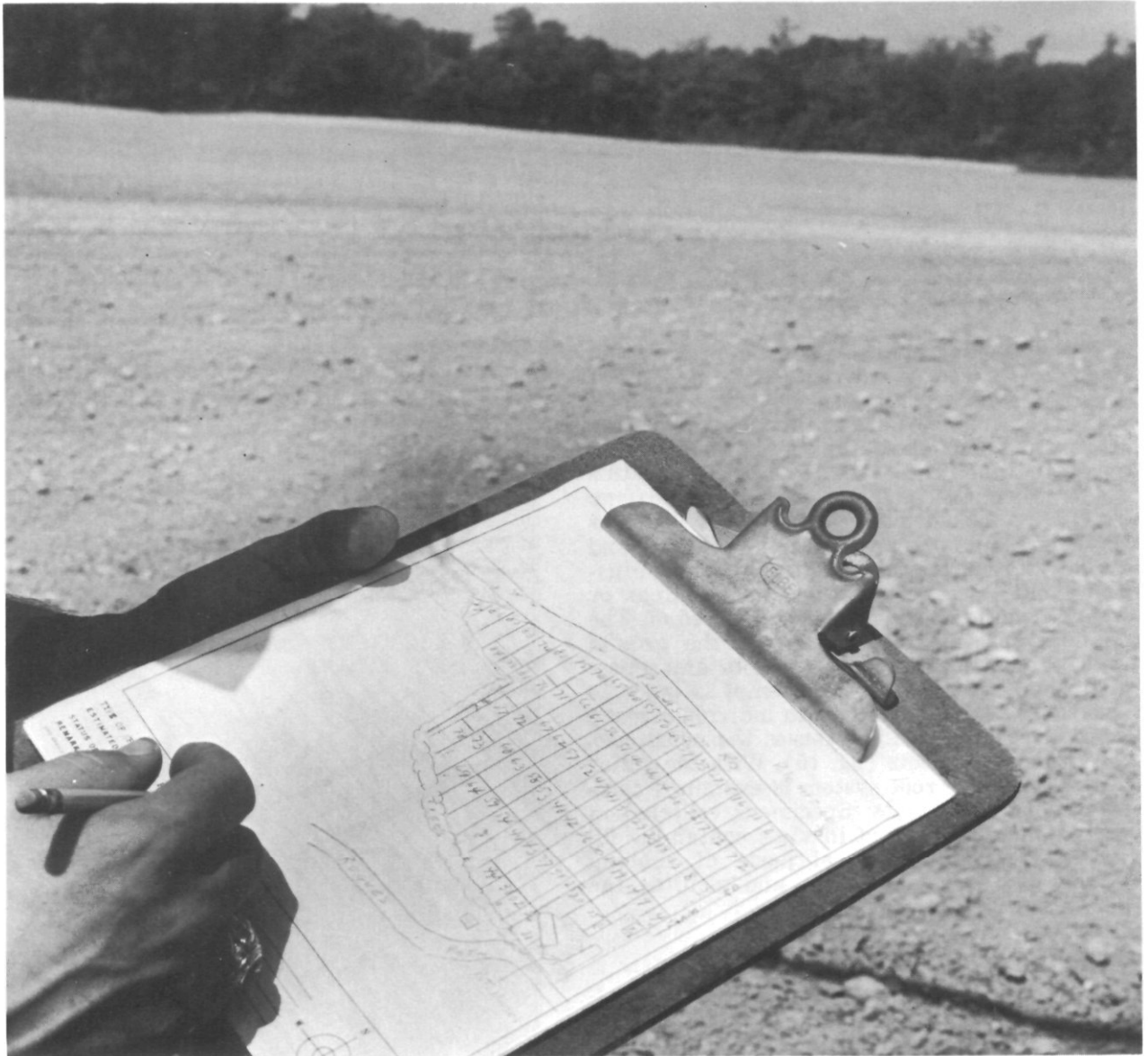
FIGURE 17.—A sketch should be made of the field to show the property location, land marks, and location in the field from which each sample was collected.
