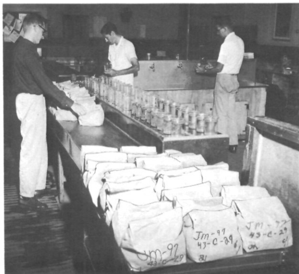
FIGURE 22.—Soil samples are washed and residues placed in beakers. Identity of every soil sample must be maintained throughout the laboratory processing.
