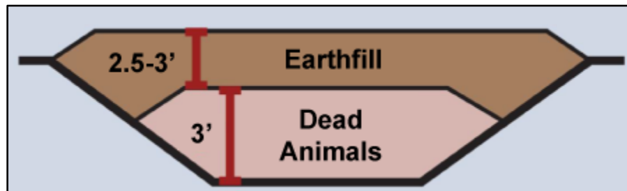
Figure 2. Illustration of Trench Configuration with Side Slopes
